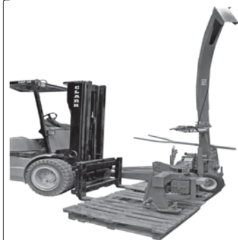
Figure 2- Transporting the machine by Forklift and Palette
